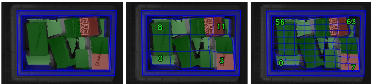
Fig. 6.6: Visualizations of the load carrier filling level: overall filling level without grid (left), 4x3 grid (center), 8x8 grid (right). The load carrier content is shown in a green gradient from white (on the load carrier floor) to dark green. The overfilled regions are visualized in red. Numbers indicate cell IDs.
