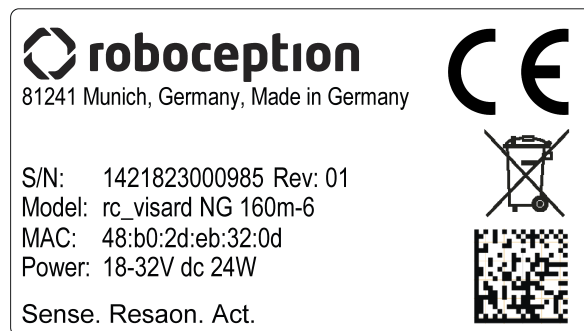
Fig. 4.1: Label on the rc_visard NG indicating model, serial number and MAC address
