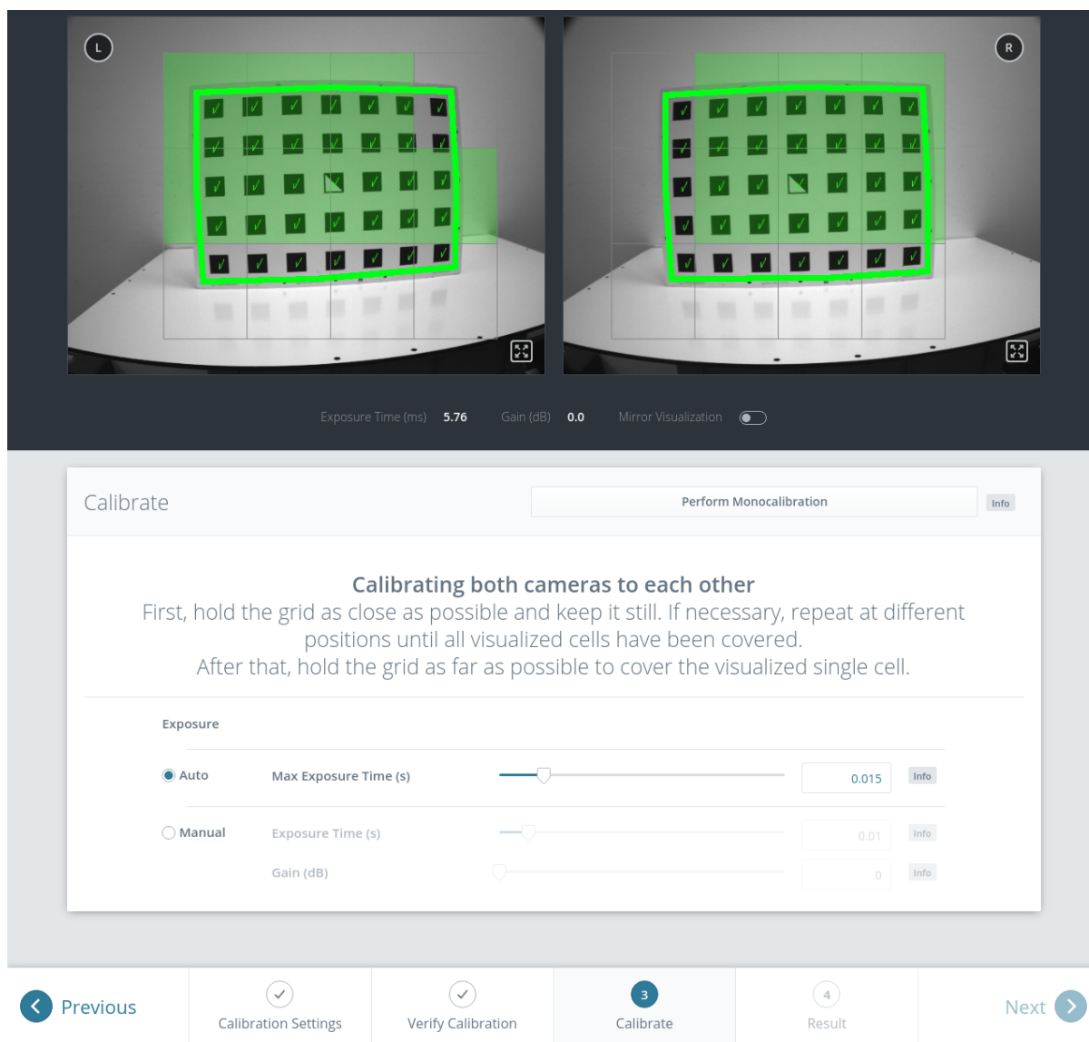
Fig. 6.30: Stereo calibration: Hold the grid as close as possible to fill all visualized cells
