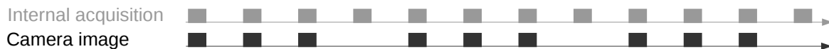
Fig. 6.2: Images are internally always captured with 25 Hz. The fps parameter determines how many of them are sent as camera images via GigE Vision.
